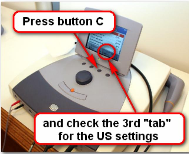
In order to start the US treatment, push button C. The 3<sup>rd</sup> "tab" will highlight and you can set the intensity of the US treatment.
